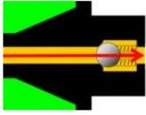
Injection material entering the one way ball valve chamber pushes the return ball towards the end of the chamber. After injection the residual pressure or the spring pushes the return ball back against its seat and stops undesired material loss.
